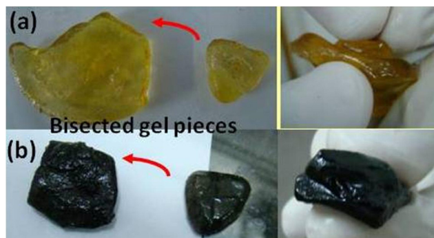
Fig. 1. Self-healing of bisected (a) guar gum-BmimCl ionic gel and (b) guar gum-BmimCl/MWCNT nanocomposite gel.
